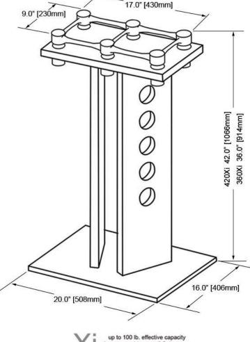
up to 100 lb. effective capacity inserts provide up to 6.5 degrees of tilt upward or downward
