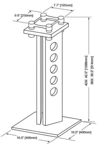
up to 75 lb. effective capacity inserts provide up to 6.5 degrees of tilt upward or downward
